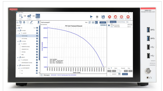
Figure 11. Forward biased I-V characteristics of solar cell measured by 4200A-SCS Parameter Analyzer.
